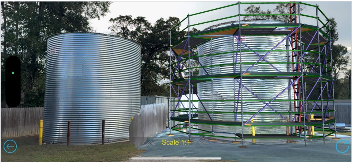
The actual structure (left) viewed with the digital twin and scaffold (right) on a mobile device in the field.
